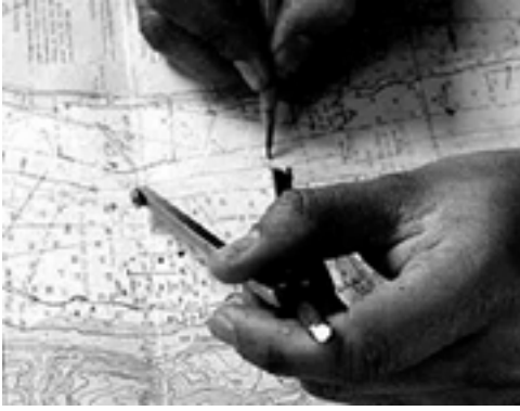
Figure 1. Using the dividers to span the distance between successive position fixes.
