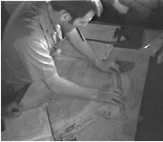
Figure 3. The positioning of the body of the plotter while adjusting the second LOP slightly clockwise. The left thumb acts as a pivot while the right hand slides the hoey arm slightly toward the plotter’s body.
