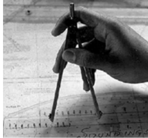
Figure 2. Transferring the spanned distance to the scale where the span may be read as either a distance or a speed depending on the way the spanned space is embedded in the navigator's activity.
