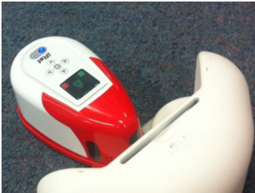
Fig. 1. iRat with its docking station. The iRat monitors its battery levels and returns to its docking station for recharging when necessary.
