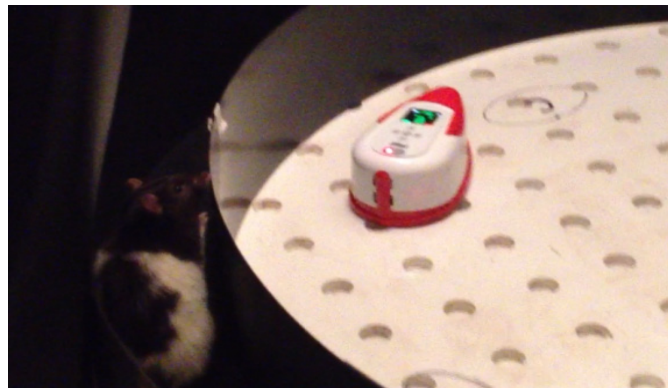
Fig. 1. iRat with its docking station. The iRat monitors its battery levels and returns to its docking station for recharging when necessary.
