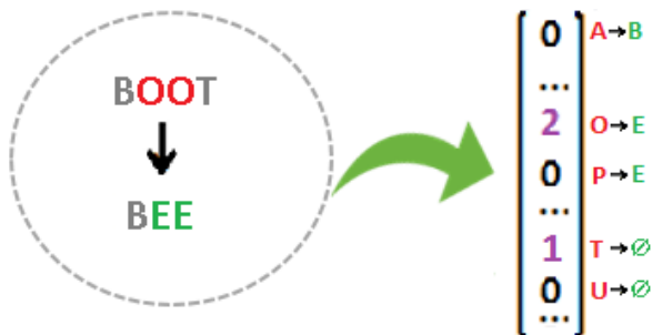
Figure 1: Each element in \nu_{ij} (the vector at left) represents a type of edit. The entry \nu_{ijm} represents the number of edits of type m that occur as string s_i ( boot ) is transformed into string s_j ( bee ).
