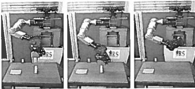
Fig. 12. Three frames extracted from the “grasping to take” sequence executed by the robot. “Taking” consists in placing the object into the box inside the robot.
