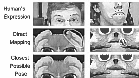
Figure 8. Noise in the neural network output and correction by Leo's motor system. The figure shows the human's expression, the neural network's direct mapping of this expression onto Leo's joint space, and the initial closest pose to this mapping in Leonardo's posegraph. The areas circled indicate joint positions in the direct mapping that are not possible for the physical robot to achieve. By using the robot's closest basis pose as the starting point for the search-to-match process, Leonardo avoids attempting to execute impossible joint configurations.
