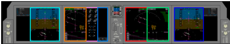
Figure 12. The seven areas of interest (AOIs) defined on the Boeing 787 Dreamliner instrument panel.
