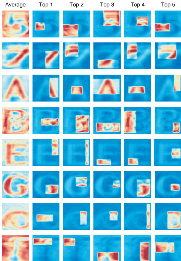
Figure 7: Visualization of the learned templates on ICDAR03-CH dataset. The first column shows the average images of each character class (from top to bottom: 5, 7, A, B, E, G, c, f). Each row shows the top K most informative sub-regions for that character class. Red and blue colors denote different image intensities from high to low. Notice that the learned top K sub-regions capture the most discriminative parts for each class.
